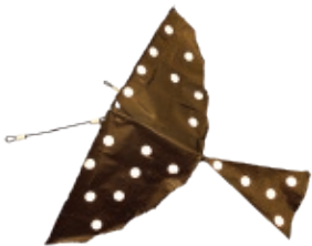
Reflective Marker Patches For mass-sensitive targets
